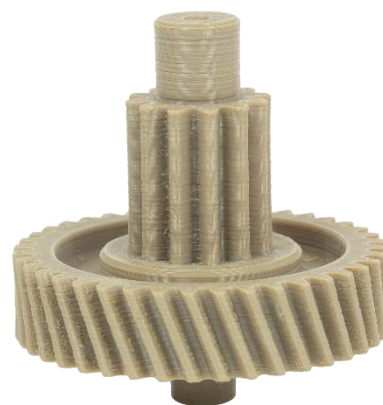
Fig. 7 Model in the semi-crystalline phase after annealing
