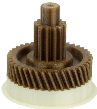
Fig. 6 Model in the amorphous phase before annealing
