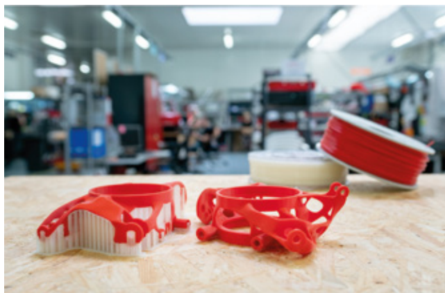
Steering knuckle was 3D printed in two parts with the use of 3DGence INDUSTRY F340.
