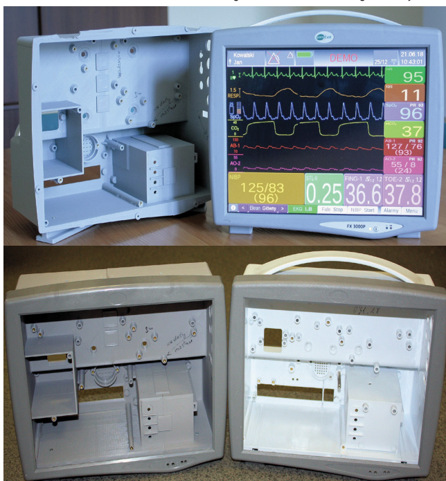
On the left - a printed housing model. On the right - the molded casing from injection.
